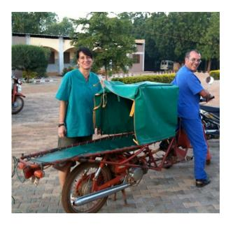
The Moto ambulance available at the hospital of Nanorò; the prolonged chassis of a Yamaha 125 on which a stretcher is placed, symbol of a population capable of adapting the solutions to the needs of the environment. Low running costs, efficiency, security, greater speed in comparison to any other means including off-road vehicles on those roads that are difficult to drive on.
